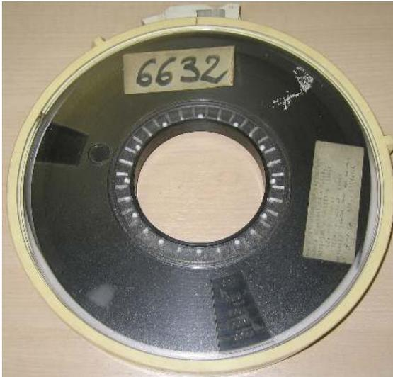
These tapes could store 5MB to 150MB of data and marked an evolutionary step in data storage and data protection. Data was initially stored on tape and later on disk. Data was copied to a “backup tape” for safe storage. Tapes were rotated in a “Son, father, grandfather” retention policy. Tapes were often moved offsite to provide a disaster recovery capability.
